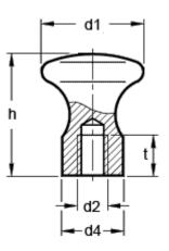
$\begin{array}{ll} d1 &= 32 \\ d2 &= M8 \\ d4 &= 18 \\ h &= 37 \\ t \mbox{ min} = 12 \end{array}$
